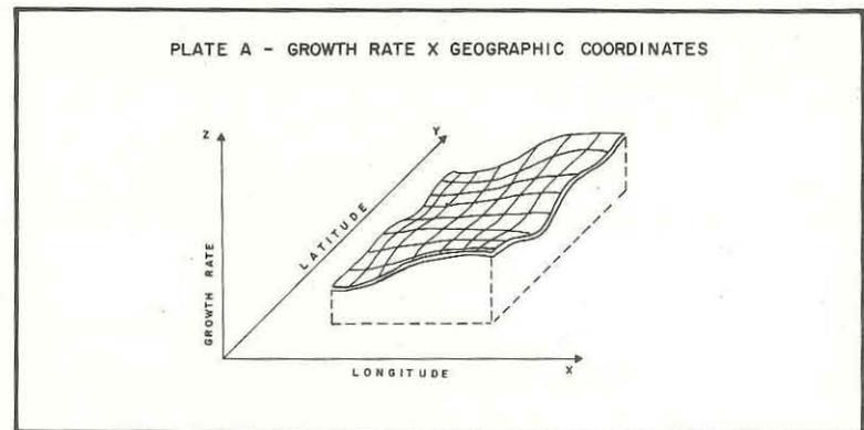
A form of simplification may be the calculation of the plane representative of the surface under consideration, using the method of least squares:
