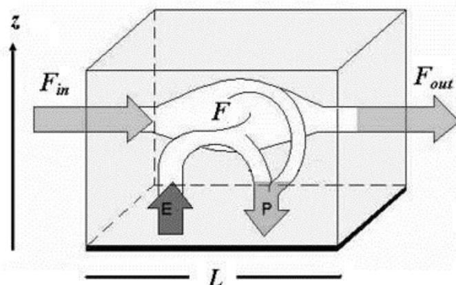
**Figure 1:** Conceptual diagram of the processes considered in precipitation recycling: total precipitation  $P$  ( $\text{mm day}^{-1}$ ), evapotranspiration  $E$  ( $\text{mm day}^{-1}$ ), average water vapor flux ( $\text{kg m}^{-1} \text{s}^{-1}$ )  $F$  where  $F_{in}$  and  $F_{out}$  are the vertically integrated water vapor fluxes ( $\text{kg m}^{-1} \text{s}^{-1}$ ) that enter and leave the area respectively of scale of length  $L$  (km). Source: Adapted from Brubaker *et al.* (1993).
